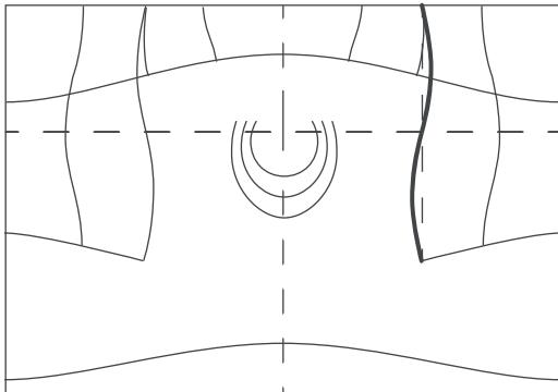
**STEP 1: mark point A (sleeve depth) to shoulder intersection (pivot at point A to align)**
